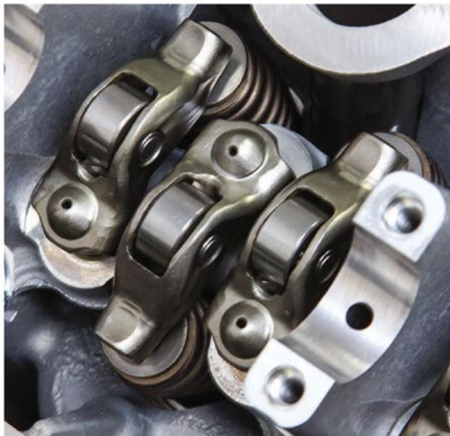
BELOW: These are the three roller followers (rocker arms), three per cylinder, that actuate two intake valves and one exhaust. These are the original 3V followers, which have the large oil holes that bleed off oil pressure and starve the oiling system, which can cause engine damage.
