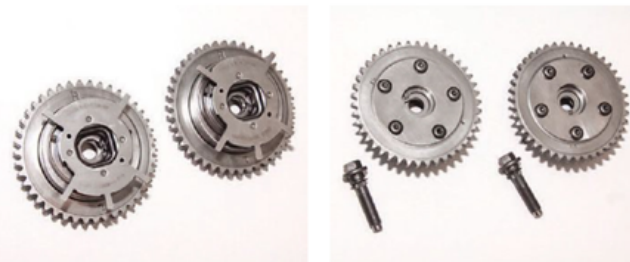
These are the revised cam phasers currently available from Ford with engineering refinements that make them more durable. Oil pressure is applied to the phaser, which advances valve timing for power under acceleration. A watch spring-style return spring retards timing back to center. The drive pins tend to fail in the original 3V phasers.
