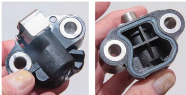
ABOVE: One of two plastic/composite timing chain tensioners, which are controlled with engine oil pressure to keep timing chains firm against the guides. The iron tensioners (not pictured) have ratchet mechanisms to lock tension in with or without oil pressure.
