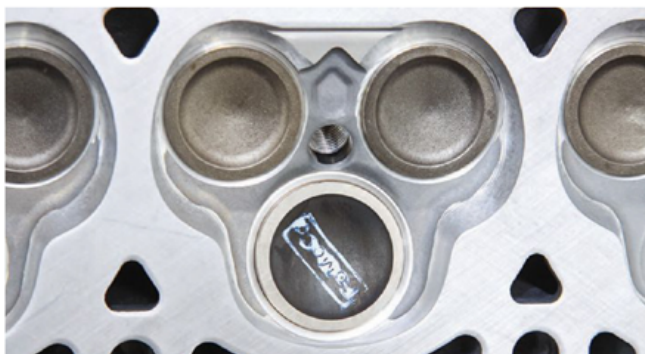
ABOVE & BELOW: The 3V cylinder heads are radically different than the 2V and 4V castings. Where they differ most are the unique three-valve chambers with two intake valves and one exhaust, with the spark plug in the middle for a thorough light-off and less chance of detonation. The 3V's block is virtually the same as the 2V offering the same rugged durability.
