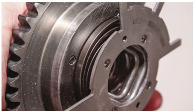
This is a close-up of the cam phaser return spring, which is one weakness in the original cam phasers. The spring fails and the cam phaser doesn't return to center.
