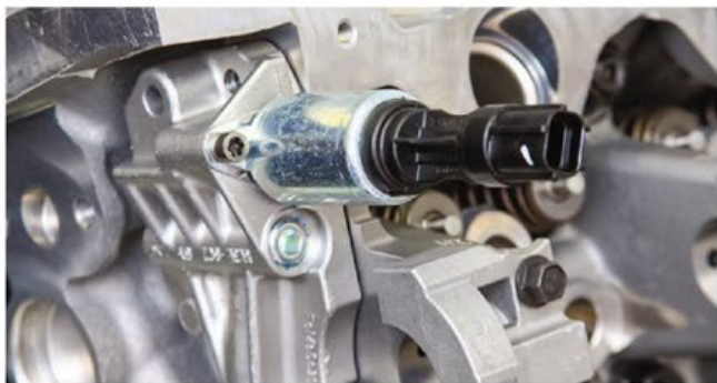
This is the VCT advance solenoid (there are two, one for each bank), which is signaled by the PCM to advance cam timing. These solenoids can stick, causing engine roughness and power loss. They stick primarily with engines that don't get regular oil changes. You must run 5W30 synthetic engine oil even though Ford suggests 5W20, which is not thick enough. Mobil 1 synthetic is suggested along with a Wix or Ford Motorcraft filter.
